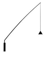
Light source: 2700K CRI >80 1041 lm 116 lm/W Fixture: 830.69 lm 92.29 lm/W Driver included: CC - Constant Current 350 mA 110~240V 50/60Hz
